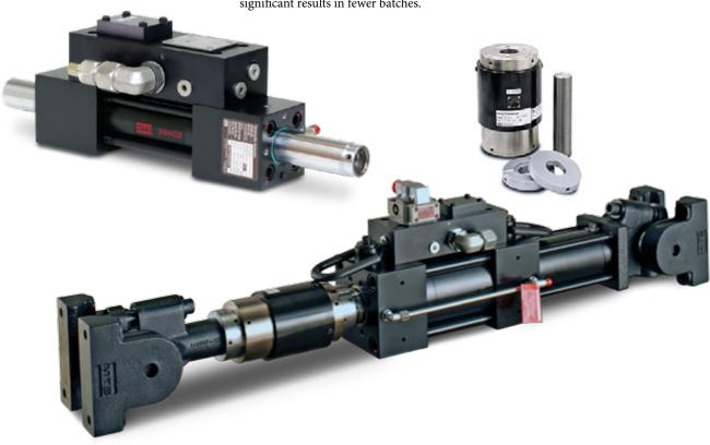
MTS DuraGlide 244 Actuators are double-ended, fatigue-rated and designed with proprietary materials that minimize friction, while maximizing reliability, wear resistance and ease of maintenance. They are hydraulically-powered pistons that can extend or retract (double-acting) to provide displacement or force into a test article or structure.
