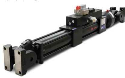
These actuators come in a greater variety of standard stroke lengths to meet a wider range of fixturing dimensions. They are available from 100-500 mm (4-20 inches, in 2-inch increments) and with force ratings from 15-1000 kN (3.3-220 kip).
